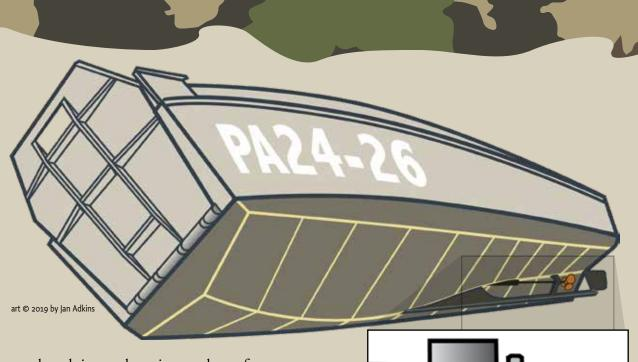
as though it were hovering on the surface. Aerated water was now pushed out the sides from under the boat before it ever reached the propeller. Not only did this allow the propeller to rotate in completely solid water, but obstacles were pushed out of the propeller's path as well. What an amazing discovery! Andrew named this new boat the Eureka.
