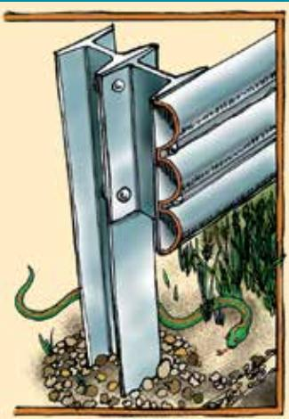
A three-beam guardrail has a piece of steel that ripples in three C-shapes. This type of guardrail is used on roads with a lot of truck traffic. The curves in the C-shapes absorb energy in a crash, and the rail is high off the ground to catch trucks.
