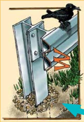
The ground that holds the posts is also very important. Engineers use math to make sure that the rails, posts, and ground together can absorb enough energy to stop a moving car safely.
